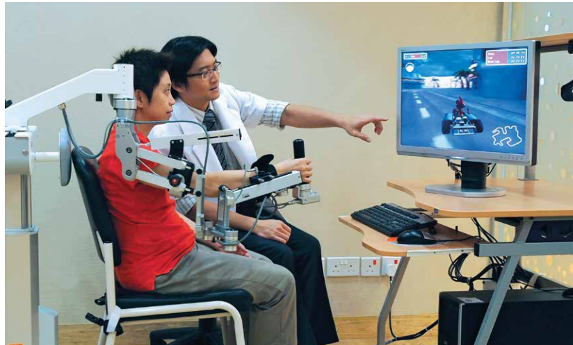
The Armeo Spring is a single-arm exoskeleton that simultaneously trains arm movements and grasp functions.
