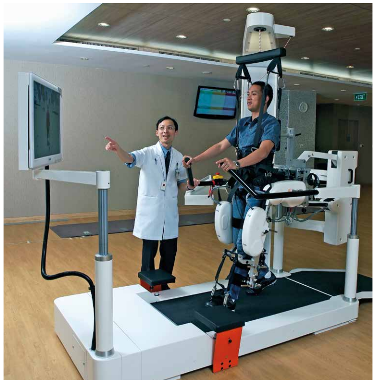
The Lokomat is a robot-assisted gait training system that straps patients into a harness while they practise walking on a treadmill.
